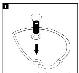
Remove all components from drain piece including: thin and thick silicone washer, hard washer, drain nut and tail piece.
