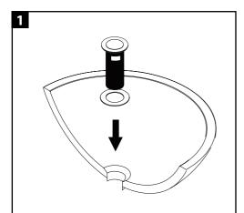
Remove all components from drain piece including: thin and thick silicone washer, hard washer, drain nut and tail piece.
