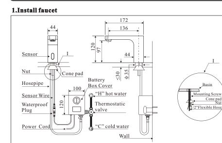
a)Fix the flexible hose and mounting screw into the faucet body.
