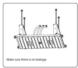
Connect the hose to pre-installed G1/2 water outlet, Open water and flush the pipe. Then connect the hose to shower body, check if there is any leakage. If leakage then fix it, If not then move the next step.
