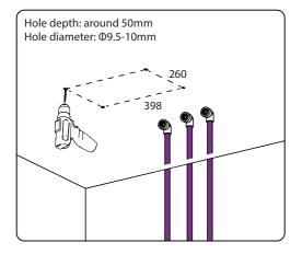
Use the bracket frame as temperate, marking the installation line by pencil. Drill 9.5-10mm diameter hole, depth around 50mm, then knock in the screw plug.
