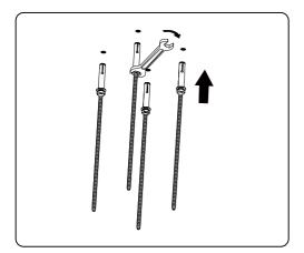
Install and tight the M6 expansion rod by using 10mm spanner
