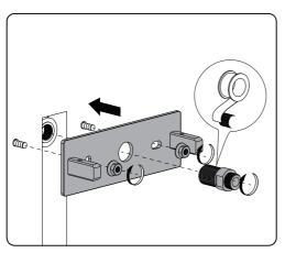
Use the removed nut and washer to install the mounting base onto the wall and tighten it. Wrap the G1/2 to G3/8 adapter's G1/2 end with Teflon tape, and use a wrench to screw it into the wall pipe.
