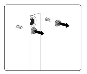
Remove the nuts and metal washers from the metal anchor and set them aside for later use.
