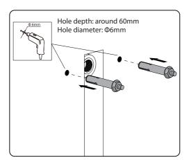
Drill holes at the marked positions with a diameter of  $\Phi$ 6mm and a depth of 60mm. Insert the metal anchor into the holes.
