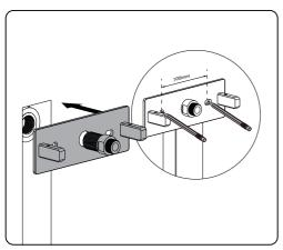
Use the mounting base and adapter as a template, use a pencil to mark the locations on the two mounting holes where drilling is needed. The center distance between these two marks is 100mm.
