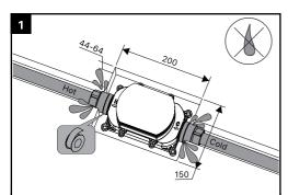
Connect the pipe to the water port, left (H) for hot water and  $\operatorname{right}(C)$  for cold water. Open the water and test the leakge.
