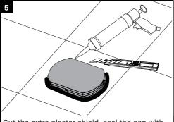
Cut the extra plaster shield, seal the gap with waterproof sealant.
