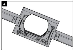
Fixing the box by cement or other filling materials and get the tiles cutted according to the box cover dimension.
