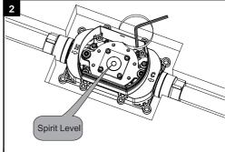
Adjust the 4 screws on valve, make sure the spirit level is at horizontal position.
