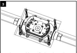
Use the screw driver to fix the valve to the floor by the screws provided.
