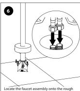
valves from floor, and secure the connection of inlet supply lines to the valves.
